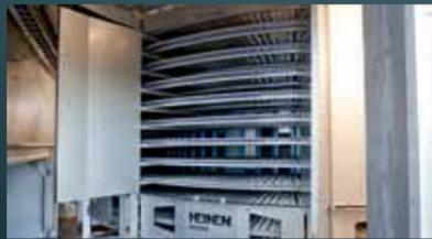
As a single or double drum system, upwards or downwards conveying, four layouts and three system diameters, and installed on the factory floor, a foundation or on a frame, the arctic meets all requirements in terms of capacity and integration in process and building.
