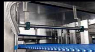
The simple belt cleaning system, with a pump unit for increasing pressure generating foam can be progressively upgraded into an extended cleaning system or even further into a fully integrated cleaning system that cleans the entire interior in addition to the belt and the conveyor system.
