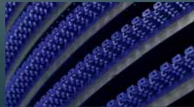
The conveyor system can accommodate a variety of different belts. Stainless steel or plastic belts, with open or closed belt surface, with small or large pitches, and with or without side plates. The stainless steel and plastic belts can be retrofitted at a later date.
